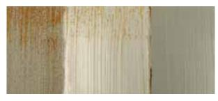
Typical brush application of traditional epoxy mastic coatings (left & centre) and Jotamastic Smart Pack (right) after continuous exposure in a salt water chamber.
